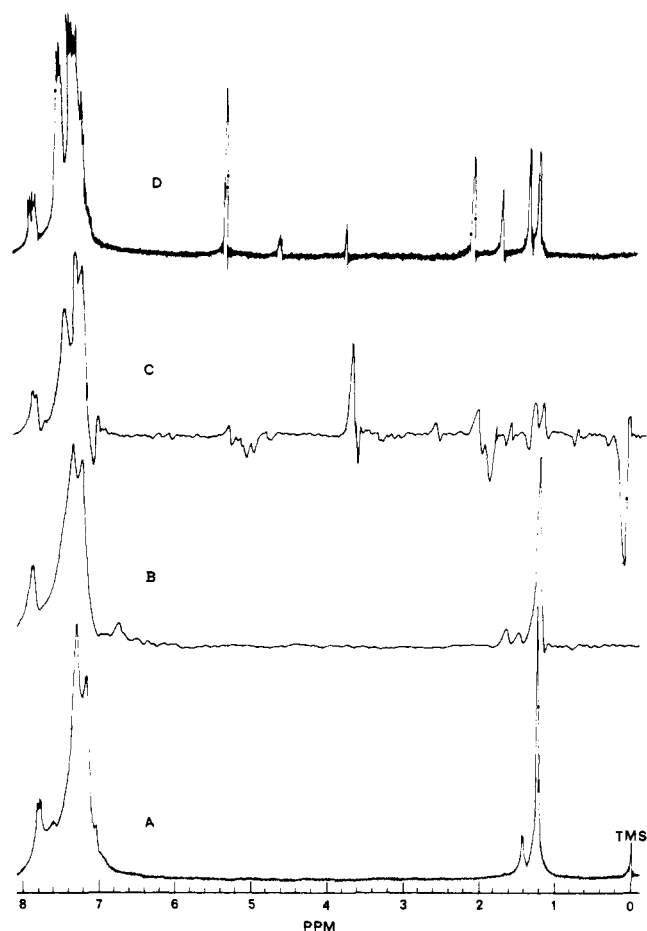
Figure 5. Representative NMR spectra of the reaction of sulfurane 1 (0.35 M) and tert -butyl hydroperoxide 6 (0.17 M) in \text{CDCl}_3 . (A) The reaction mixture at -50\text{ }^{\circ}\text{C} (slow scan at 250 s/8 ppm). (B, C) Two representative spectra at temperatures between -50\text{ }^{\circ}\text{C} and room temperature ( \sim 25\text{ }^{\circ}\text{C} ) (fast scans at 10 s/8 ppm). (D) The product mixture at room temperature (slow scan at 250 s/8 ppm).
